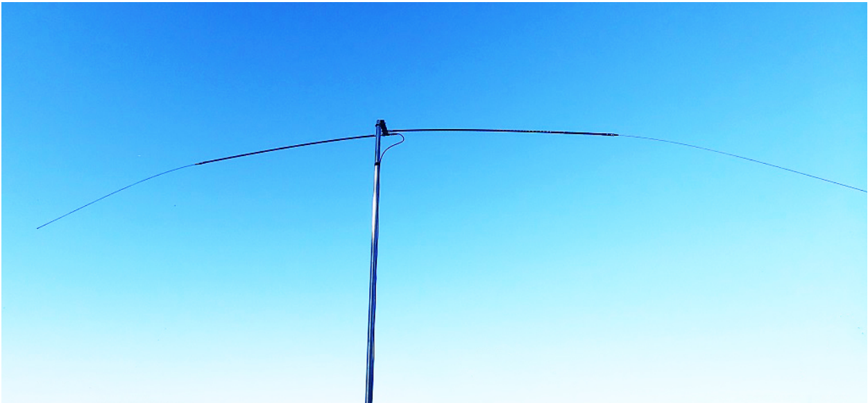
Mobile antenna dipole (2 Hamsticks)
